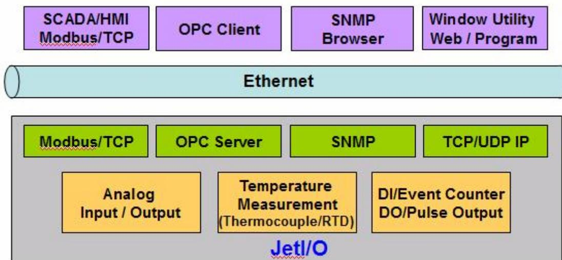
Figure 1. The Jetl/O Intelligent Ethernet I/O Server Architecture.
